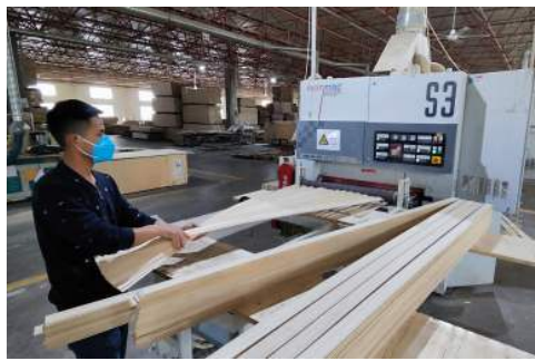
8. 确认订单后开始机器砂光 8. Start sanding slats after the order comes in.
