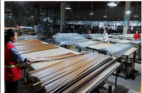
9. 手工打磨叶片边部 9. Workers hand sanding for the edge to make sure the edge smooths.
