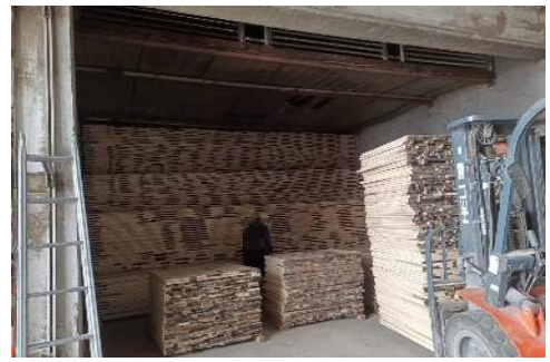
4. 意大利烘干窑技术烘干原料。 4. The drying in the Italian kiln promotes the redistribution of water in the wood.
