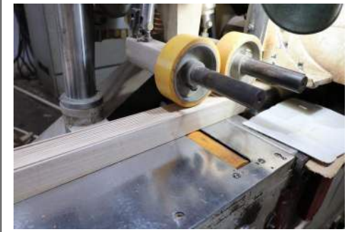
6. 木百叶专用多片锯开片 6. Enter the cutting machine for cutting slats.
