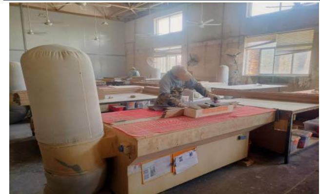
Workers hand sanding for the edge to make sure the edge smooth
