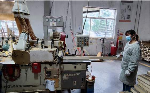
Enter the cutting machine for cutting slats,
