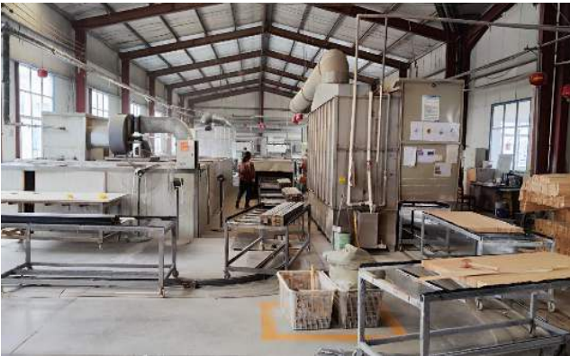
Slats enter the paint room, spray edges
