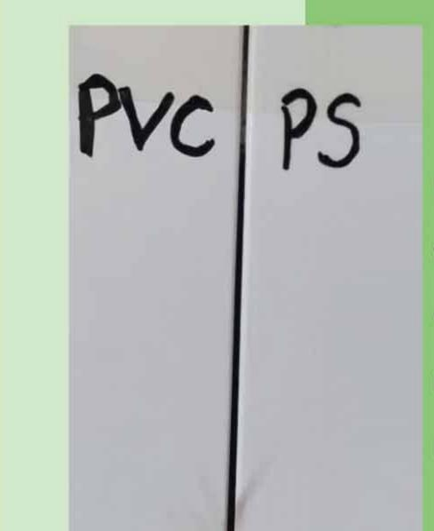
PVC: There is no flame under high temperature, and the burning stops when it is away from the fire. There is no pungent smell and no floating
