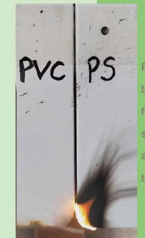
S: It burns quickly when exposed to fire, with black substances floating away and a strong pungent smell. After a small burn, a large area of black material will be left on
