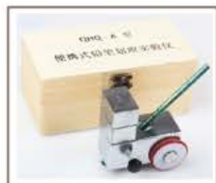
Pencil Hardness Test
